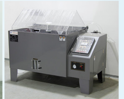
Salt mist test machine
